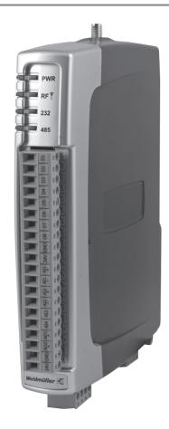
The Weidmuller WI-I/O-2-E-N wireless networking I/O and gateway is a multiple I/O node that extends communications to sensors and actuators in local, remote, or difficult to reach locations. Designed with a standards based 802.11b/g/n wireless transceiver, the WI-I/O-2-E-N can provide IP-based networking across sprawling industrial environments typical of industrial applications and includes built-in I/O capability for digital and analog inputs and outputs.
